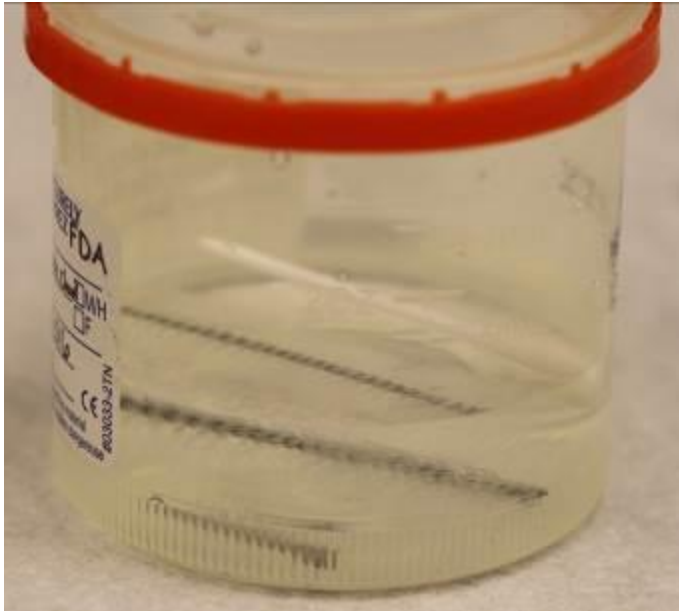
Sample container with liquid extract and swab and brush heads (prior to A5.3.6)
